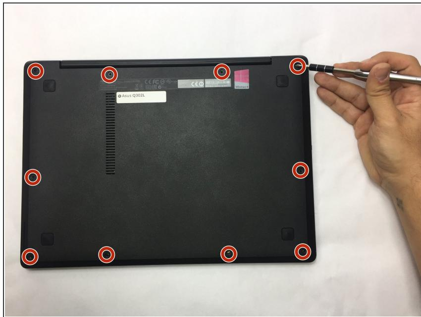
**⚠** Make sure the laptop is disconnected from a power supply and is TURNED OFF.
