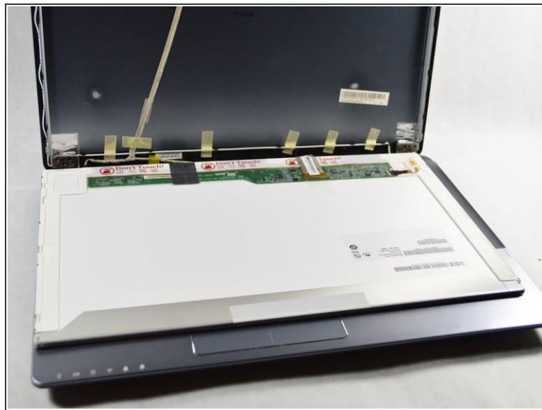
⚠ Don't tear off the bottom of the screen or you might damage the connector cable.
