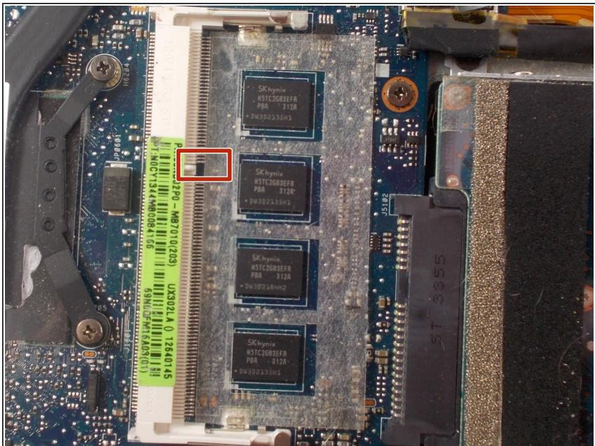
➡ To insert the new RAM, line up the hole on the RAM stick and slot.
