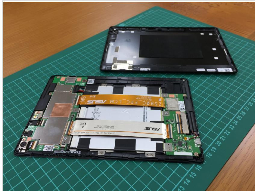
*(i)* The back case didn't use any screw or glue. The back case only use tenons to stick with front case. It's not hard to take apart.
