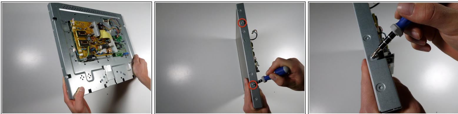
① Turn the monitor on its side so that the power supply and circuit board are facing to the right
