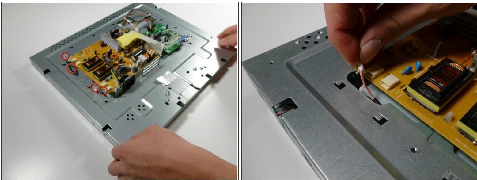
① Set the monitor back down so that the power supply and circuit board are facing you.
