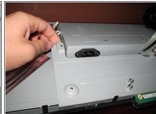
➡ Removal of the lower shield is not required but makes the job easier. ***To remove it, unclip the plastic tabs on the LCD bezel.***
