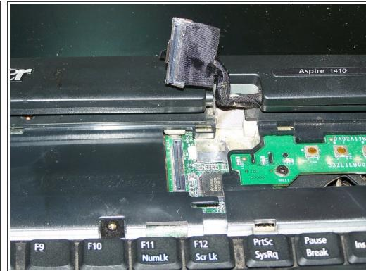
**⚠** Turn laptop over and open the screen fully. Take care as the screen is still connected to the logic board via black cable on right hinge.
