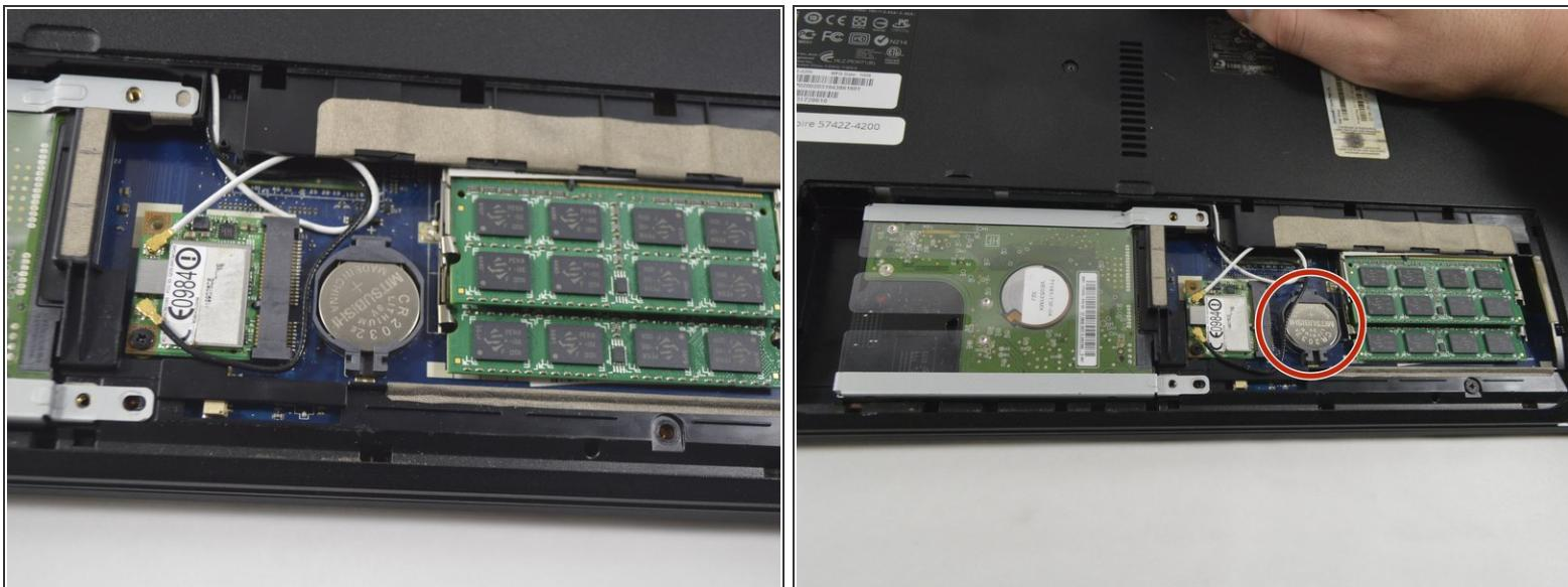
ⓘ After removing the cover panel, you will see the hard drive, the RAM, and the CMOS battery.
