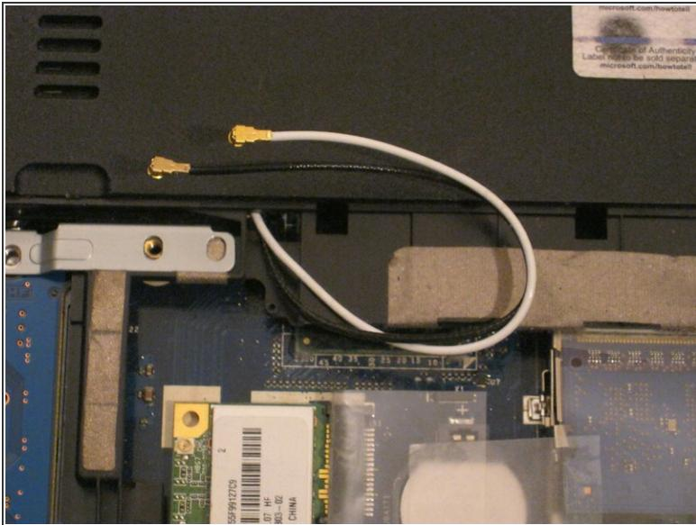
*(i)* You may find it useful to pull the antenna cables out from under the plastic retaining clip so you can move them out of the way while you work.
