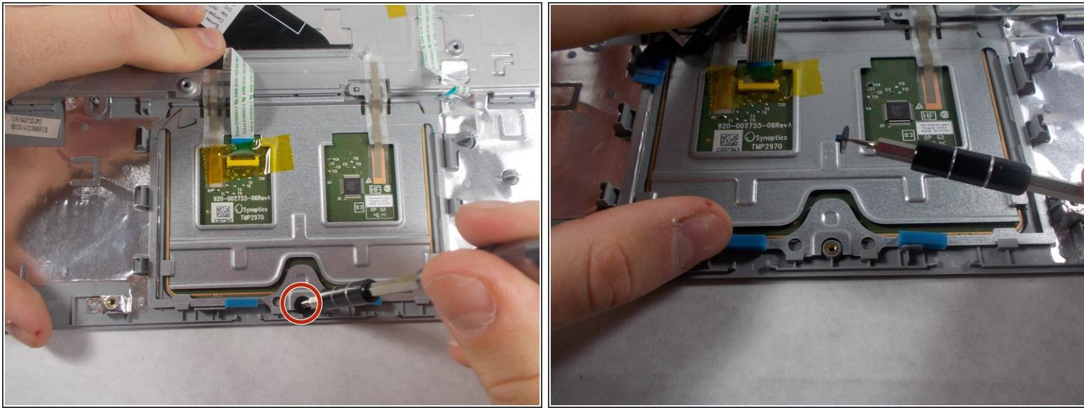
*(i)* Make sure you have removed the keyboard before attempting to remove the touchpad.
