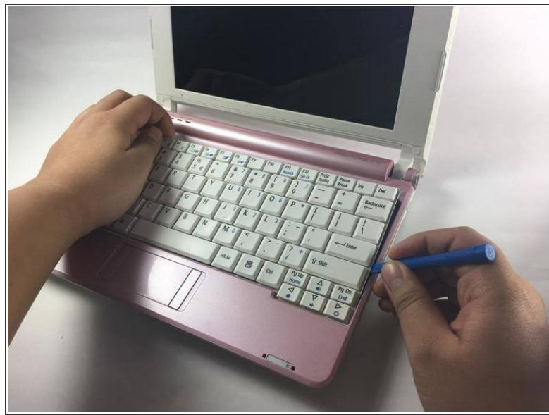
*(i)* There is a notch on the right side of the casing that blocks the keyboards ability to be removed.
