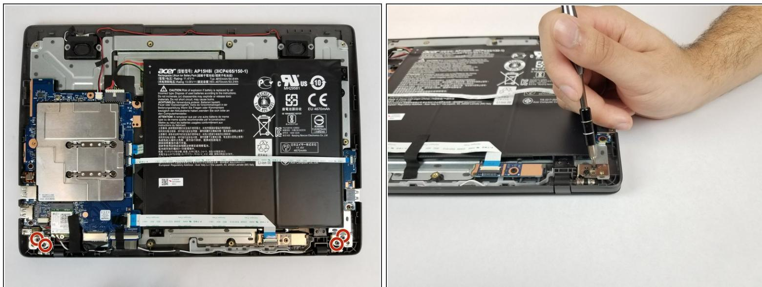
*(i)* The battery is installed in these pictures but should always be removed before any part replacement.
