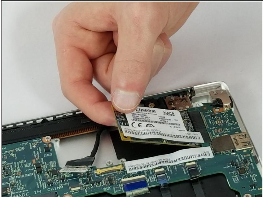
**⚠ Remove the hard drive by pulling it away horizontally from its connection.**
