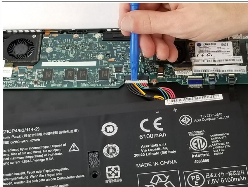
⚠ Disconnect the cable located at the top of the battery. Be careful to pull the cable horizontally, not vertically.
