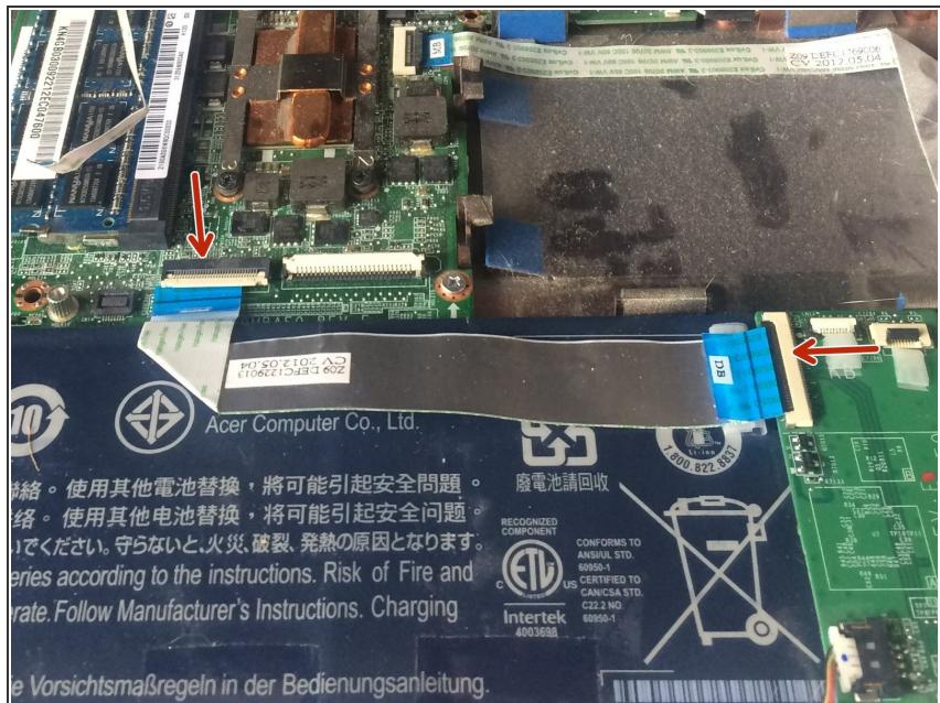
**i** After removing the keyboard, open the laptop screen to face you.
