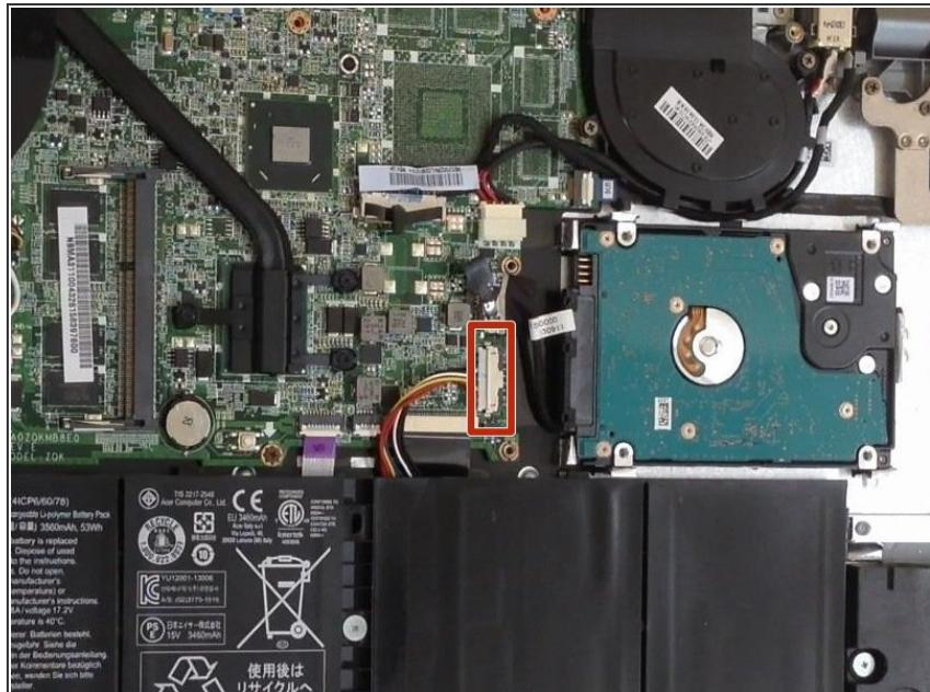
⚠ Disconnect the battery immediately for a safer repair.
