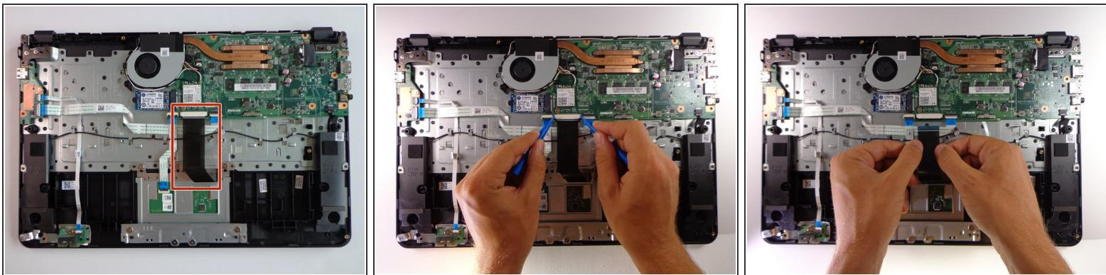
⚠ Before beginning hard drive replacement, the back cover should be taken off and the battery removed to ensure no power is connected.
