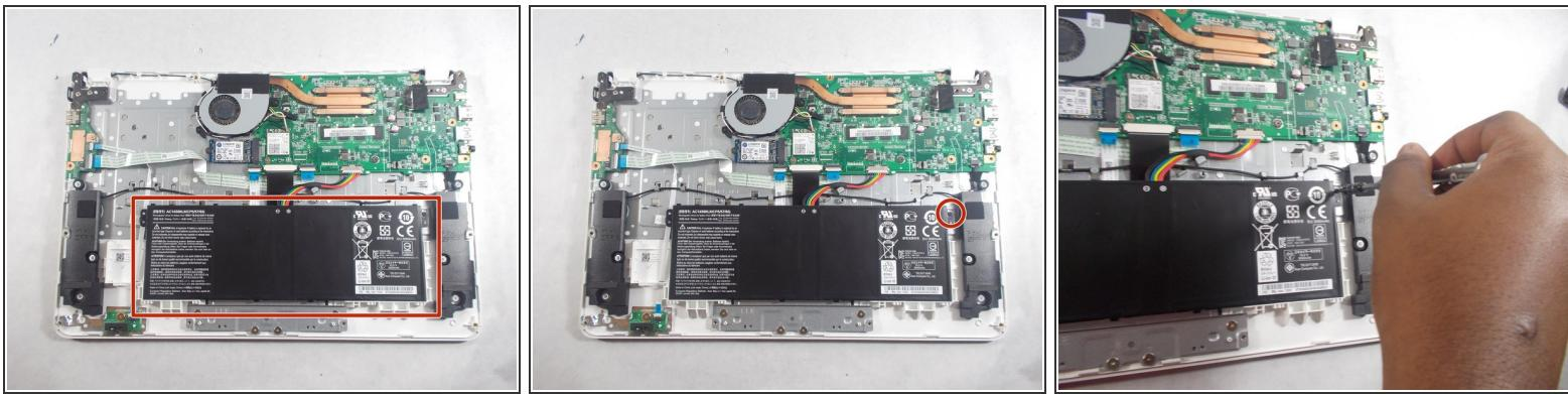
*(i)* The battery is the large black rectangle located in the bottom center of the device.
