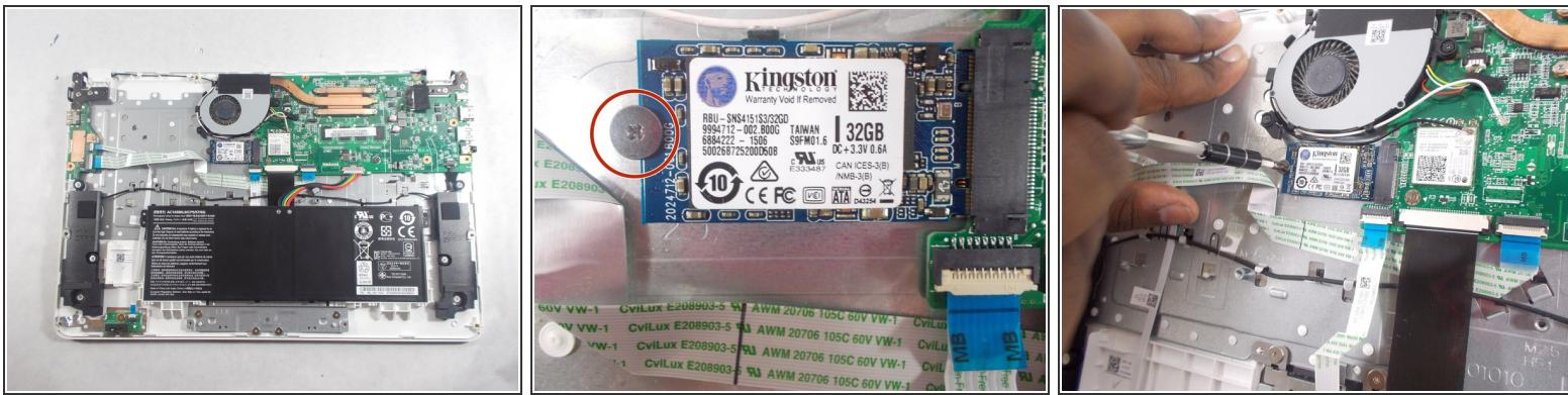
ⓘ The Solid State Drive is the blue chip locate right beneath the fan.
