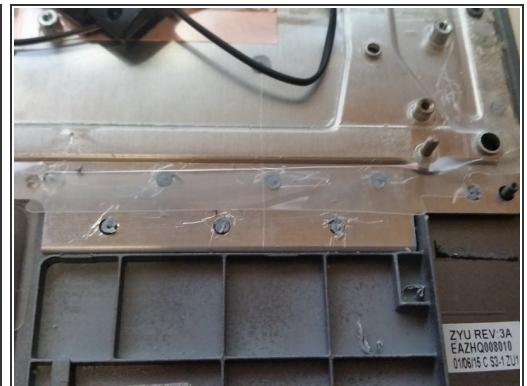
*(i)* The motherboard plate is held onto the frame by plastic pins.
