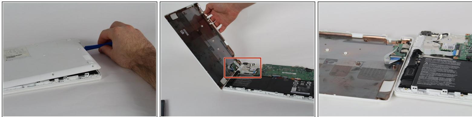
**⚠** There is a wire connecting the two pieces of the laptop, from the inside, on the left, be careful not to damage it.
