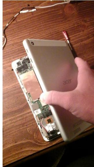
⚠ Make sure the tablet is powered off, not just sleeping, and that it is unplugged.
