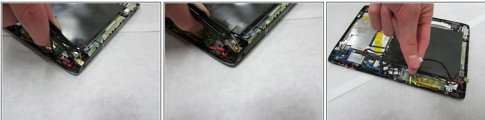
**ⓘ** The port may be taped from underneath and need a bit of force to take out.
