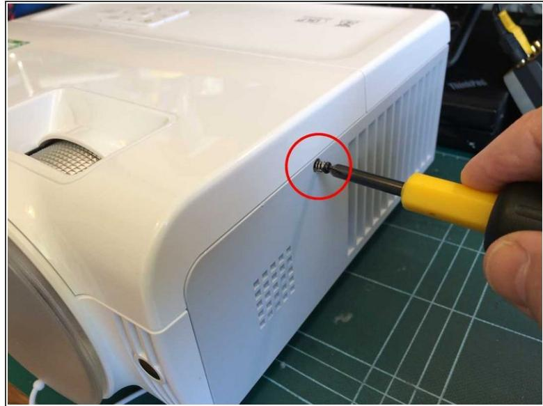
**⚠** The bulb gets extremely hot. To avoid danger of burns, do not start disassembly until the projector has been switched off and allowed to cool for at least 30 - 40 minutes.
