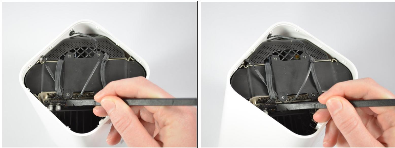
**⚠** Four black internal wires, three thin and one thick, are connected to the logic board: three by small end clips and one by a larger end clip. Handle the clips gently; they break easily.
