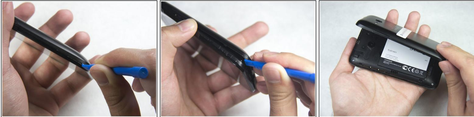
**⚠** Turn off the phone before proceeding with disassembly to prevent shock and potential shorting of any electrical components.
