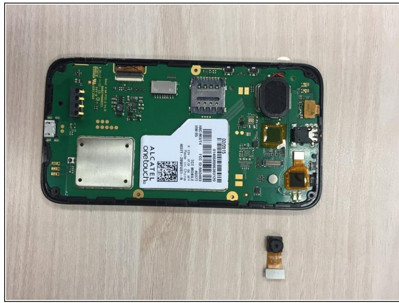
⚠ The camera should detach easily. If you are experiencing difficulty detaching it, stop and make sure the correct piece is being worked on.
