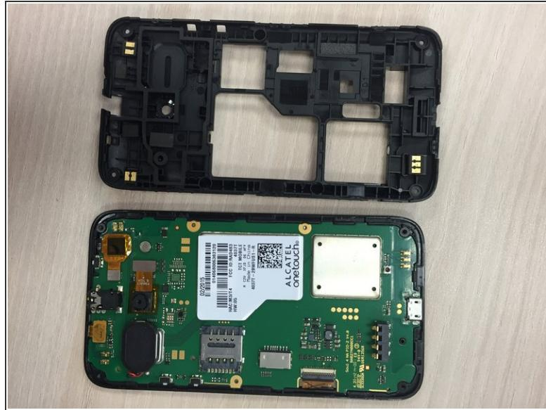
**⚠** This step may prove difficult as there are many pressure points holding the plastic backing in place. Use moderate force to pry them apart, but be careful not to snap the plastic or scratch the inside of the phone.
