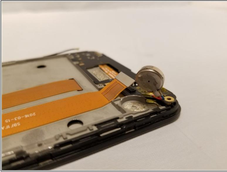
⚠ Be sure that you're reaching down far enough into the crack before you begin prying the vibrator up, or you could break it.
