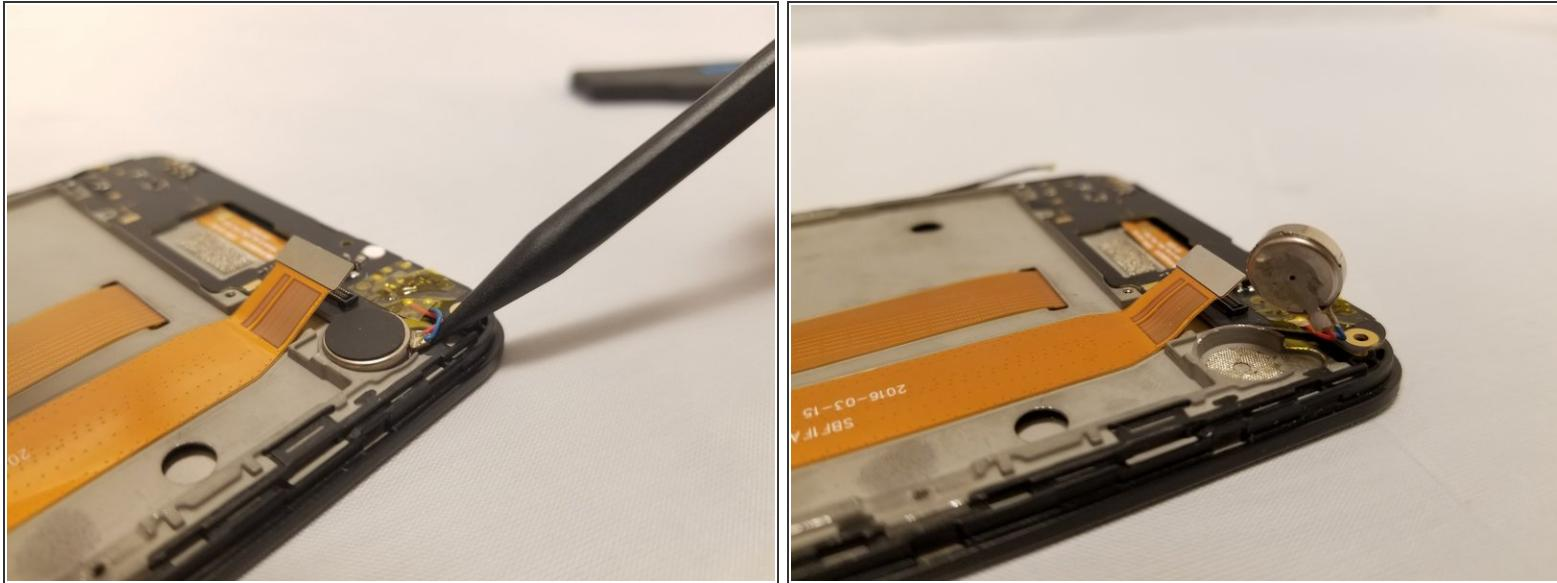
**⚠** Be sure that you're reaching down far enough into the crack before you begin prying the vibrator up, or you could break it.
