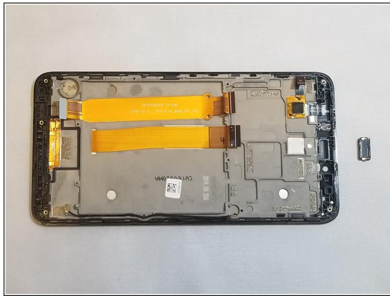
⚠ The earpiece speaker is heavily glued onto the device. Make sure you're reaching far enough down before you start prying.
