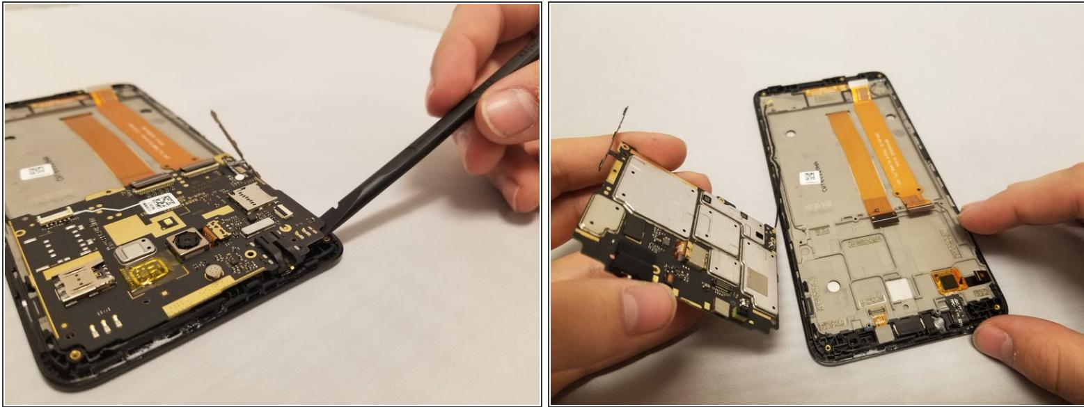
**⚠** Be wary of remaining adhesive from the volume buttons when removing the motherboard.
