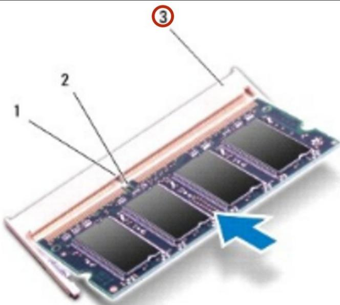
*(i)* NOTE: If you need to install memory modules in two connectors, install a memory module in the lower connector before you install a module in the upper connector
