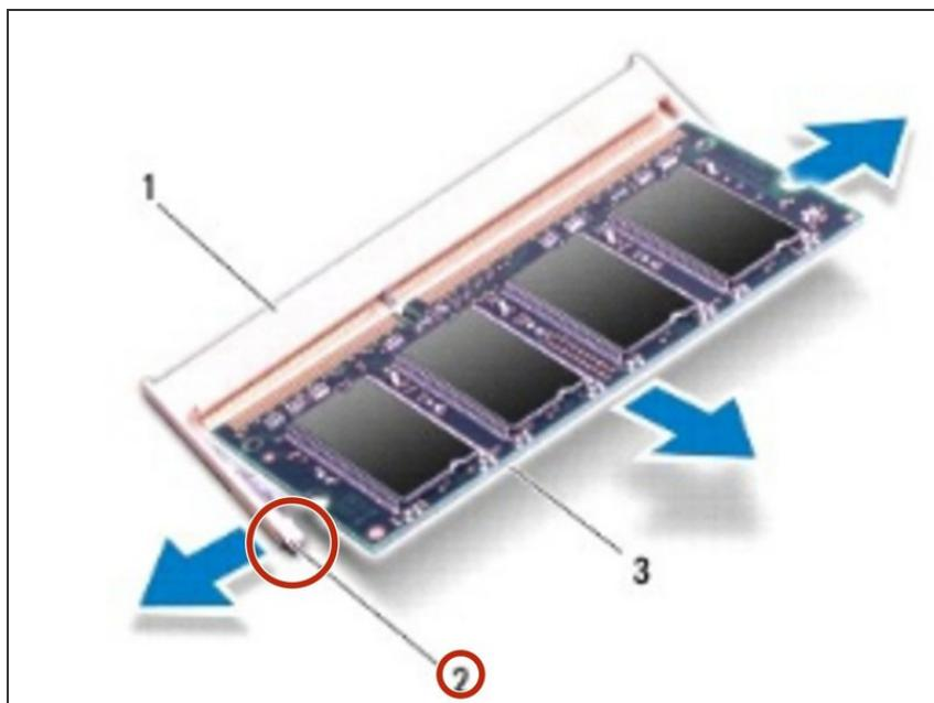
**⚠️** **CAUTION:** To prevent damage to the memory module connector, do not use tools to spread the memory module securing clips.
