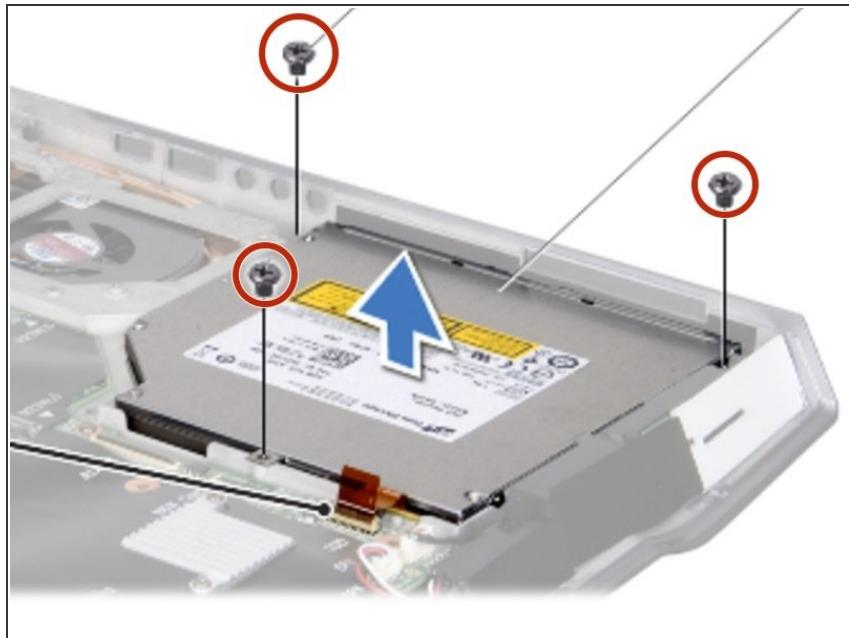
**i** Make sure the Center Control Center, Keyboard, Palm Rest, Display Assembly, Magnesium Cover and Input/Output Board is removed.
