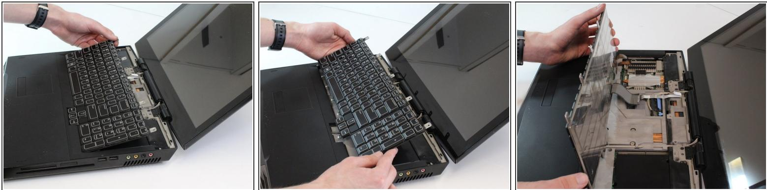
*(i)* There are two cables connected from the underside of the keyboard to the laptop.
