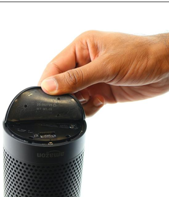
**⚠** Power off and unplug your Echo before disassembly. Failure to do so could result in injury or damage to the device.
