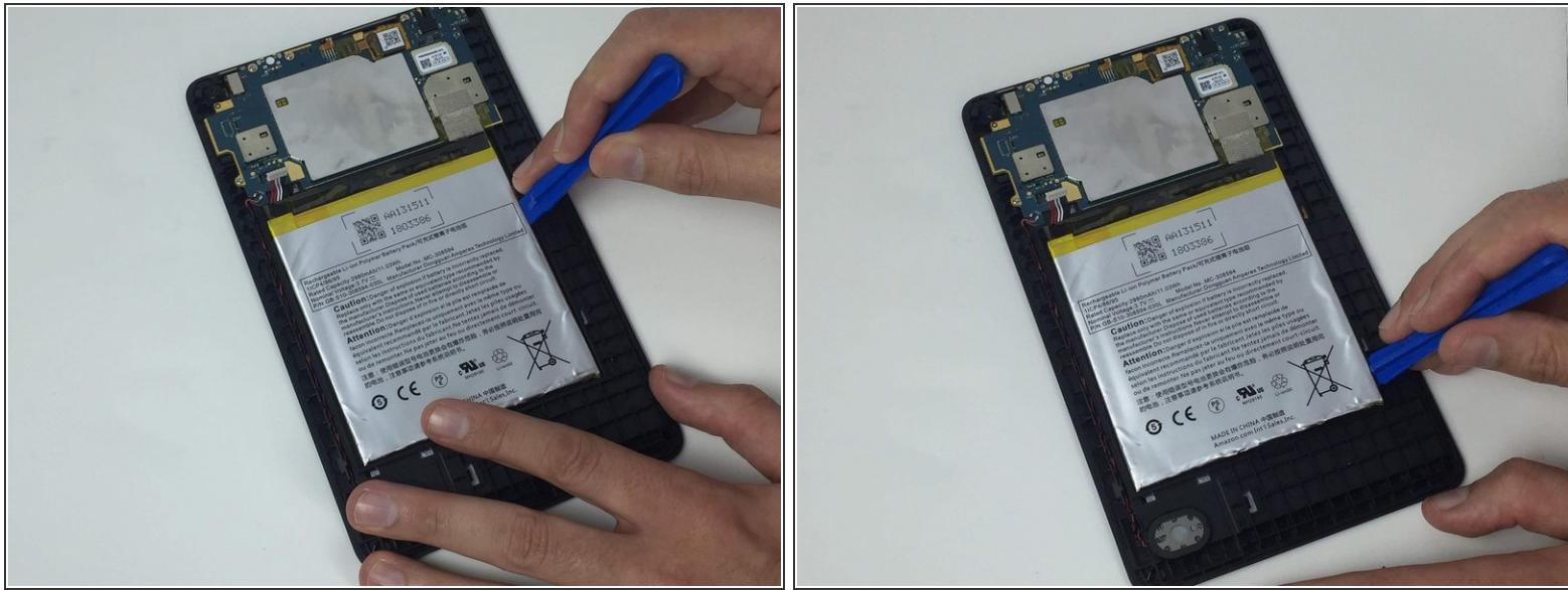
*(i)* Because heat is required to remove the screen and LCD, it is advisable to remove the battery entirely as well.
