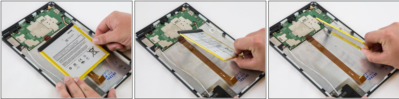
! Make sure all the adhesive is removed before trying to lift the battery from the case.
