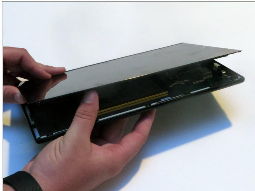
! Do not completely remove the screen yet as there is a ZIF connector connected.
