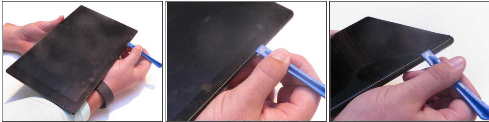
! Avoid prying near bottom right hand side due to LCD Connector
