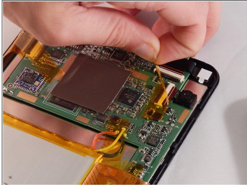
*i* The rear facing camera is located at the top right just below the front facing camera as looking inside the device.
