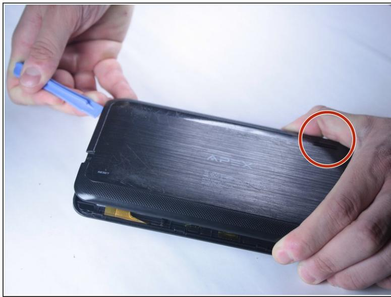
**⚠ CAUTION:** When removing the back panel of the tablet, take caution around the speaker. This is located in the lower right corner when looking at the back of the tablet. There are two wires inside connecting the tablet back panel to the device itself and this connection may be severed if the back is pulled off without care.
