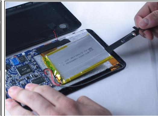
**⚠** The battery is very fragile, so this process may cause some damage to the old battery during removal. Take extra care if you need the old battery to remain intact.
