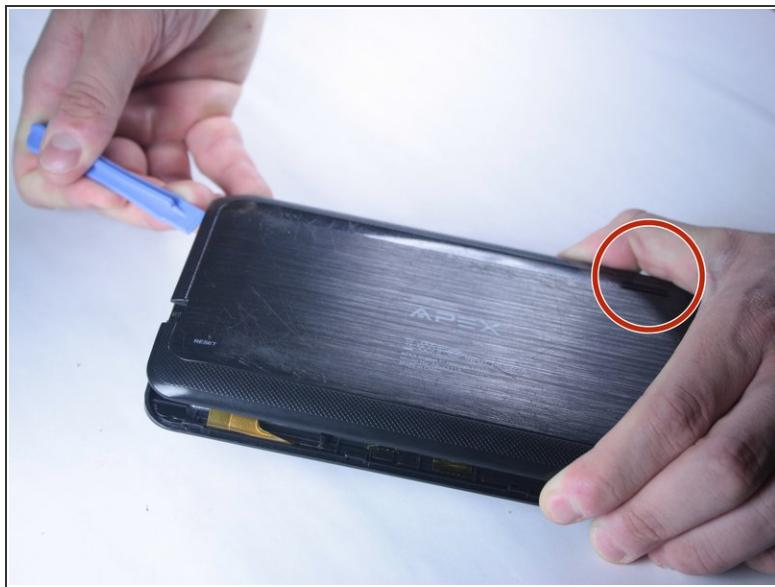
**⚠ CAUTION:** When removing the back panel of the tablet, take caution around the speaker. This is located in the lower right corner when looking at the back of the tablet. There are two wires inside connecting the tablet back panel to the device itself and this connection may be severed if the back is pulled off without care.
