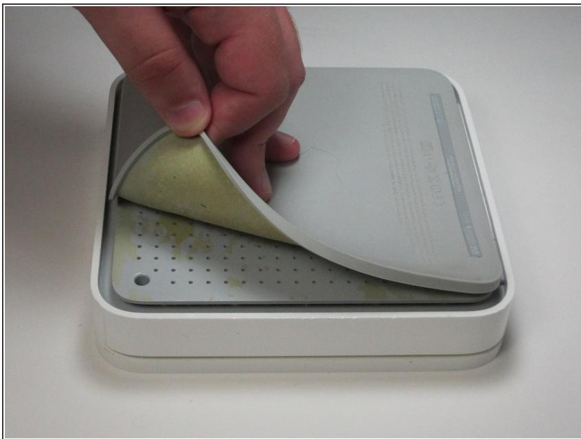
**⚠** The back pad is held in with glue so use caution when removing to prevent tearing. Low heat may be used to help remove the pad.
