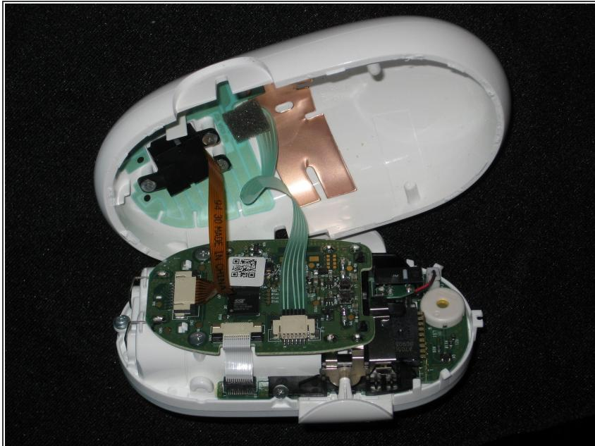
**⚠ Carefully separate the two halves; do not pull on the flex cables.**
