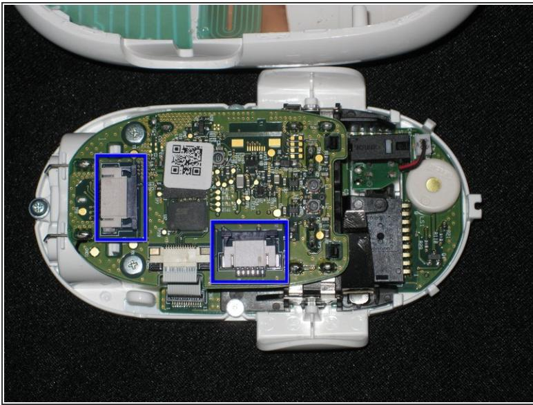
⚠ Gently unlock the latches with a fingernail or a spudger. Do not stress the latch, or it might break.
