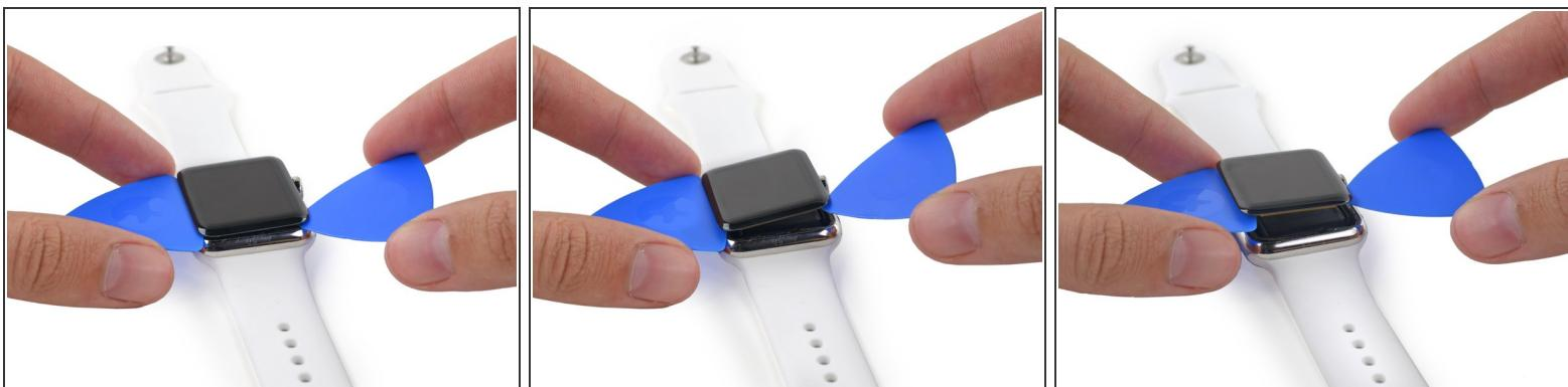
! There are two cables connecting the screen to the inside of the watch, near the top left corner. Be careful when prying or you may damage these cables.
