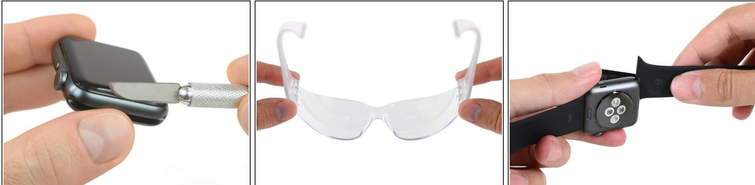
**i** Because the gap between the screen and watch body is so thin, a sharp blade is needed to separate the two. **Read the following warnings carefully before proceeding.**
