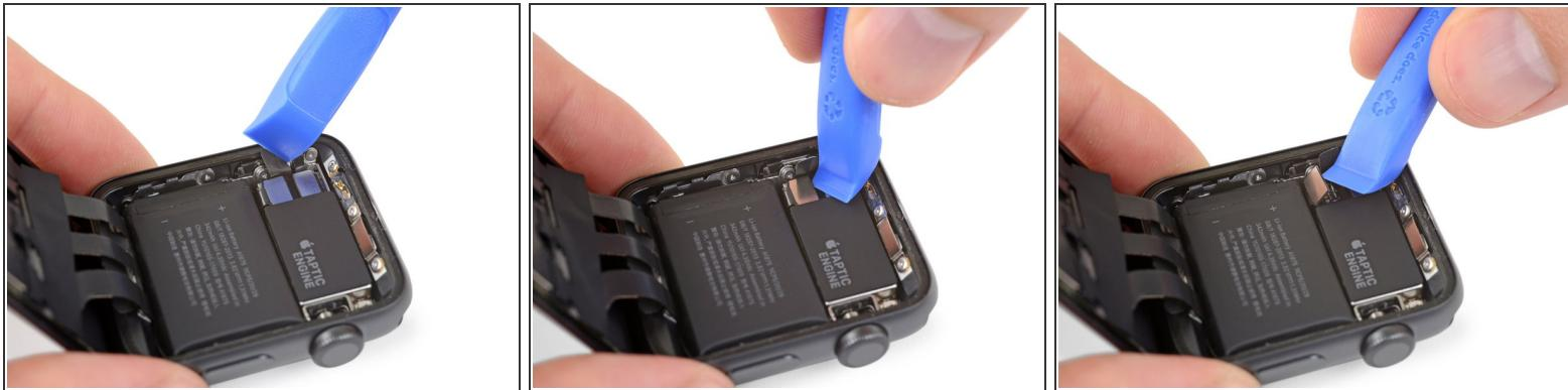
*(i)* On the GPS-only version it is possible to disconnect the battery immediately. For the cellular/LTE version, you need to disconnect the Force Touch gasket and fold it out of the way first, in order to disconnect the battery.
