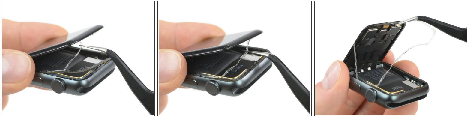
⚠ To avoid straining the display cables, don't open the display all the way yet.
