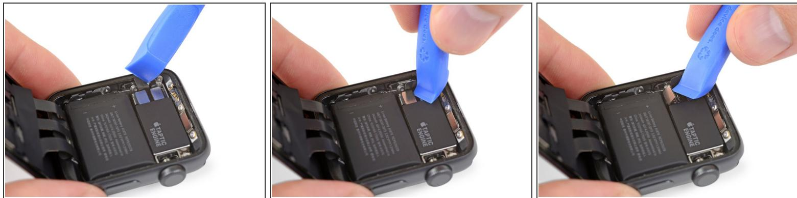
ⓘ On the GPS-only version it is possible to disconnect the battery immediately. For the cellular/LTE version, you need to disconnect the Force Touch gasket and fold it out of the way first, in order to disconnect the battery.
