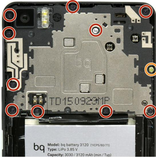
**i** Damaging the liquid indicator sticker, on the middle most screw, will void the warranty of the phone.
