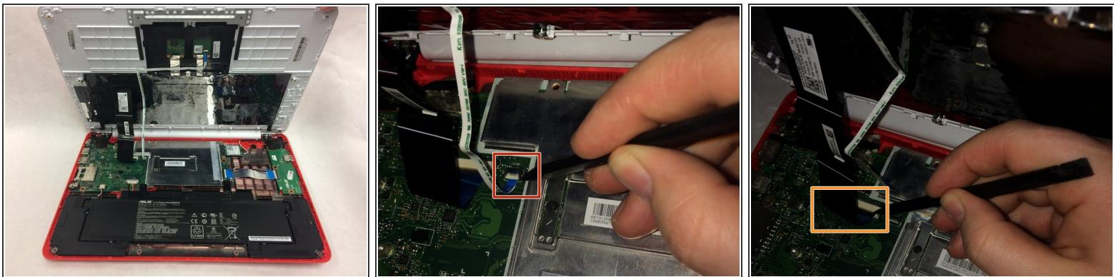
*(i)* The small and wide ribbon cables connect the keyboard to the motherboard.
