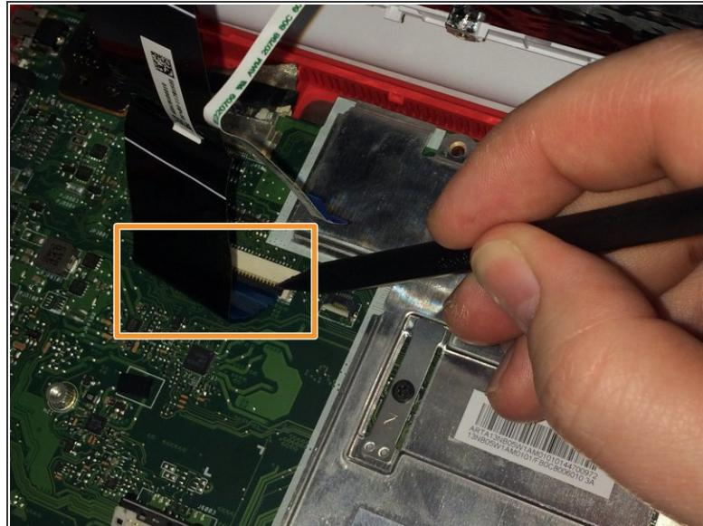
*(i)* The small and wide ribbon cables connect the keyboard to the motherboard.
