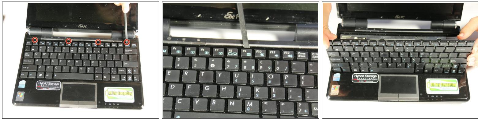
**⚠** The keyboard will still be attached to the body of the netbook at the conclusion of this step through a ribbon cable located at the bottom edge of the keyboard. Improper removal may result in damage to your device.
