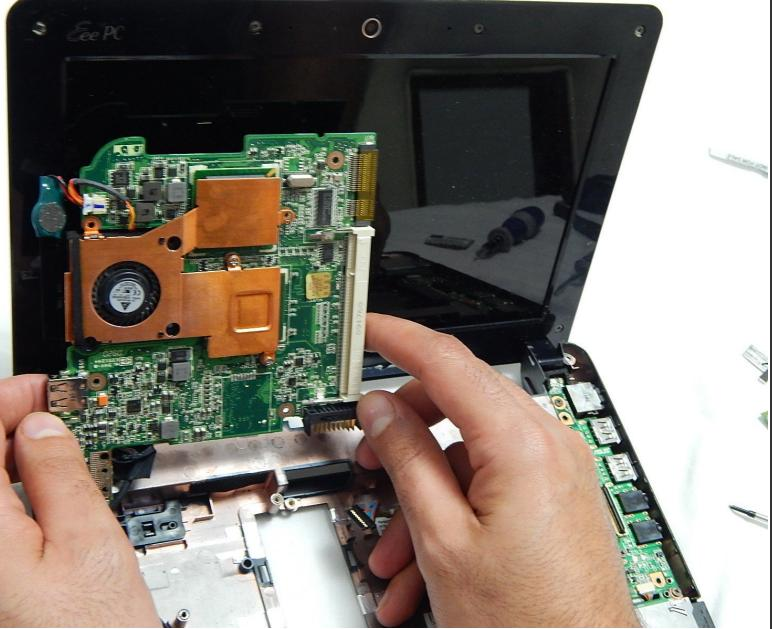
⚠ Gently lift the motherboard and hold it so that the bottom of the board is exposed.
